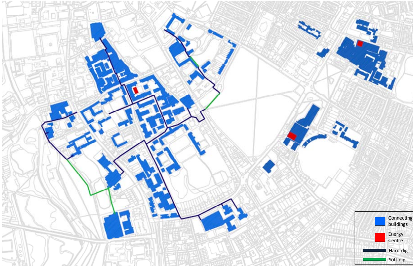
Figure 25: Map showing the Option 3 DH network covering city wide covering only the western part of the city with proposed Energy Centre in the vicinity of Downing Site. There are possibly separate schemes for the Parkside Pool area and the ARU
