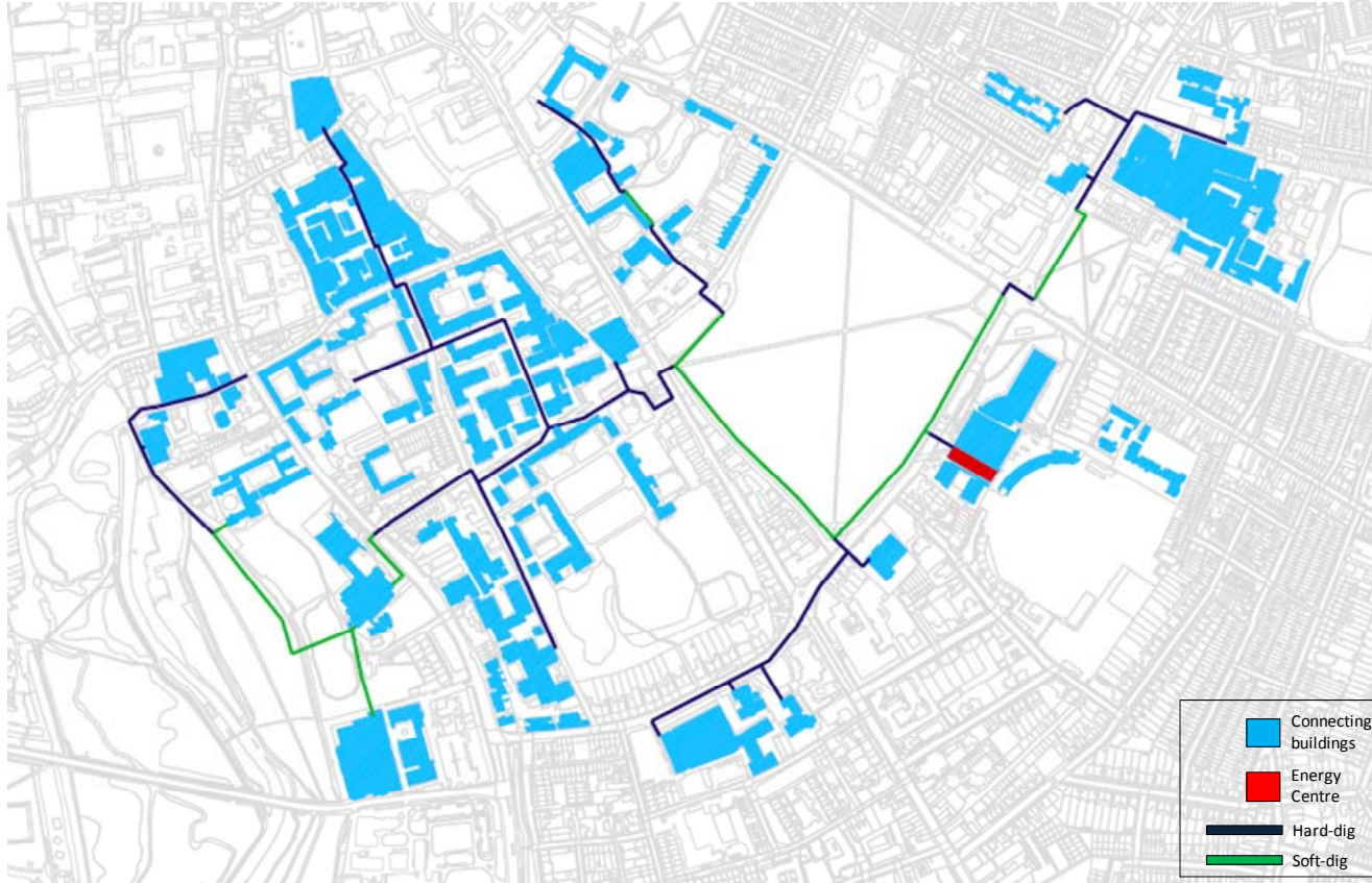
Figure 23: Map showing the Option 1 DH network covering city wide connecting the eastern and western part of the city with proposed Energy Centre at KK/QAT
